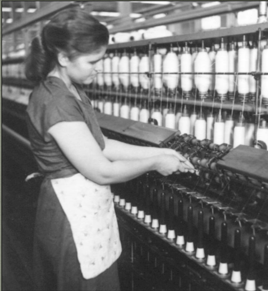
Pho-A-0688. An unidentified American Thread Company worker demonstrates the proper use of a spinning machine for a company safety brochure. Willimantic, CT, 1943. Black and white gelatin print snapshot. Unknown photographer. The worker uses a tool, rather than her fingernails, to clean lint from the machine's rollers. Most spinners were women. While few spinners suffered loss of limbs, they did experience hearing loss from the noisy machines and lung disease from inhaling cotton fibers. Later machines had vacuum tubes that sucked away most of the lint, but this machine lacks such a feature. Notice that the worker did not have a safety mask.
