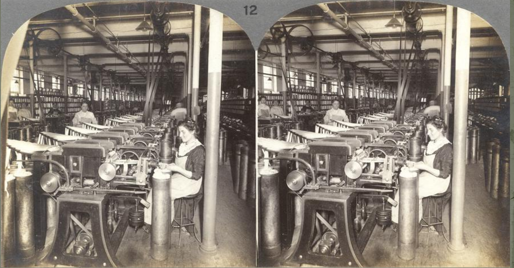
Stereograph. Unidentified workers operating drawing machines at Cheney silk mills in South Manchester, CT, 1914. Keystone View Company, Meadville, PA. The machines were powered by leather belts attached to overhead drive shafts. The drive shafts were connected in turn to waterwheels.
