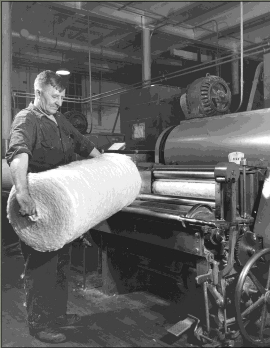
Pho-A-0381. Ignacy Pekarski takes picker lap off a picker at the American Thread Company in Willimantic, CT, c. 1950. Pickers removed unwanted materials from raw cotton and transformed it into a rolled-up sheets that could be fed into carding machines. The rolls of lap were very heavy, and most picker operators were strong men. Black and white gelatin print. Unknown photographer.
