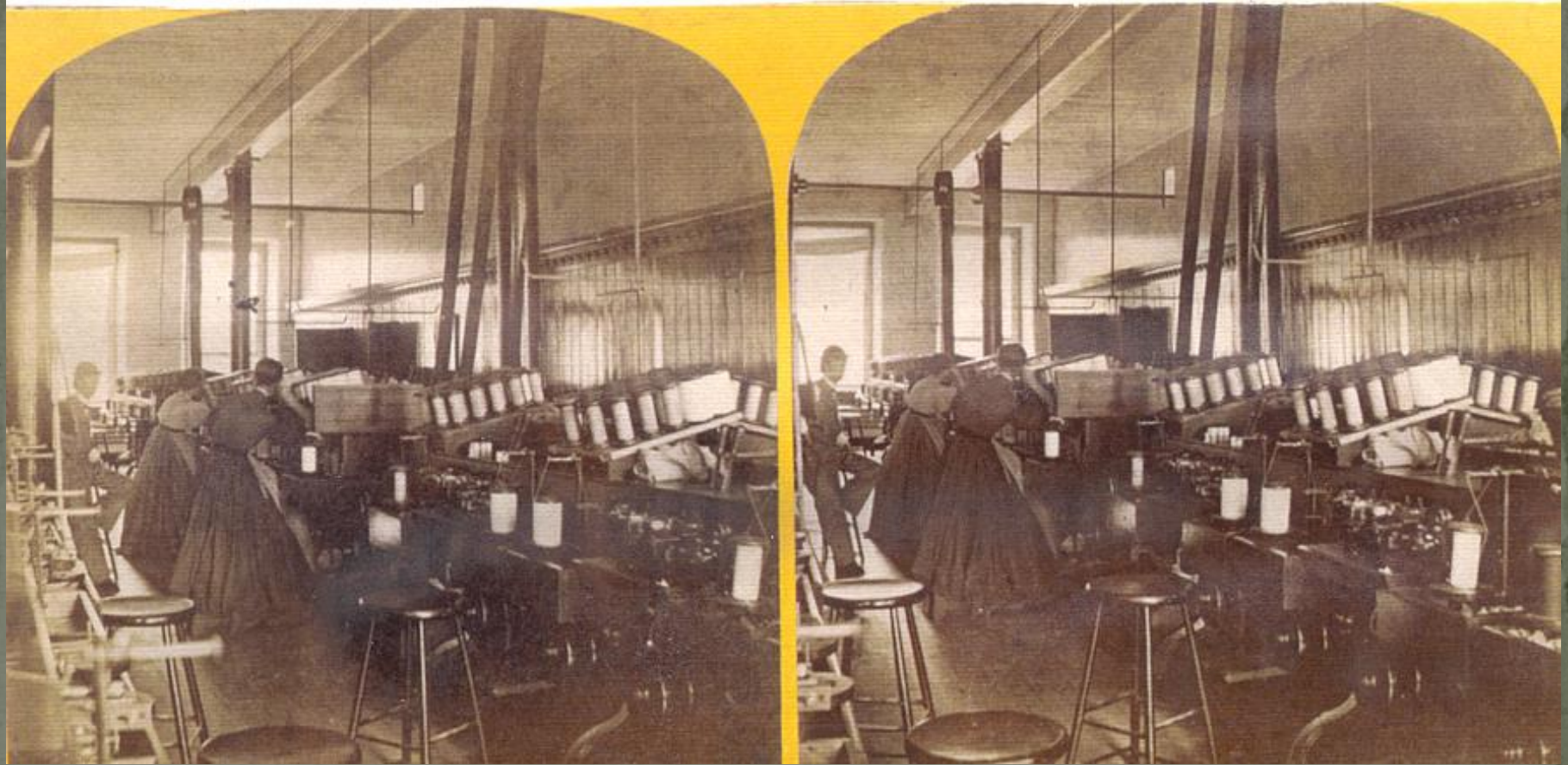
Stereograph. Unidentified workers in the winding room at the Willimantic Linen Company in Willimantic, CT, c. 1880-90. Prescott and White, photographers, Hartford, CT. Notice the long skirts. Also notice the stools – unlike most mill workers, these women apparently were permitted occasionally to sit. They would have worked about 10 hours a day. Notice the noisy leather belts that connect to ceiling-mounted drive shafts. There do not seem to be any electric lights in this mill room, indicating that work shifts still followed the rhythms of natural light. The man in the photo appears to be a foreman or supervisor.
